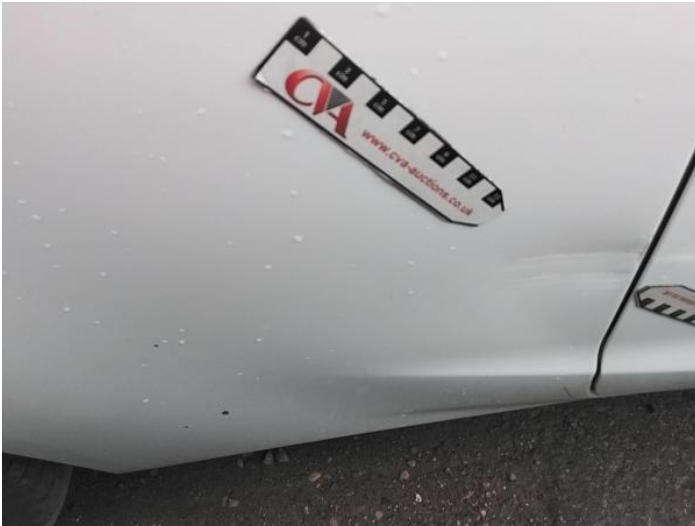
9: Qtr Panel osr Dented With Paint Damage
