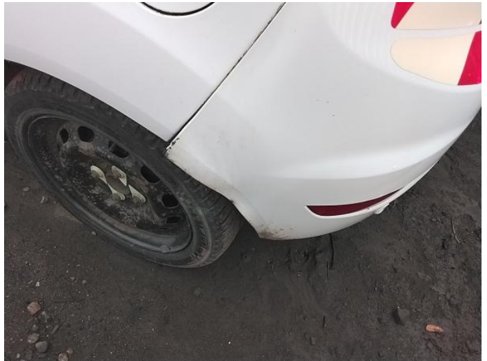
6: Bumper Rear Dented With Paint Damage
