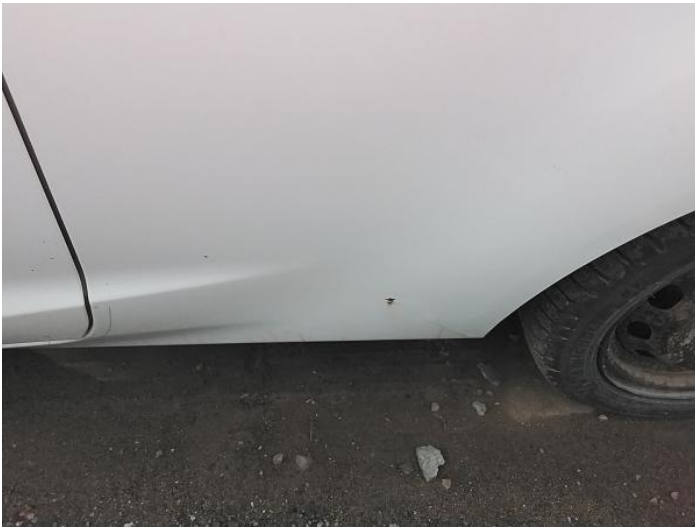
5: Qtr Panel nsr Chipped Multiple Chips
