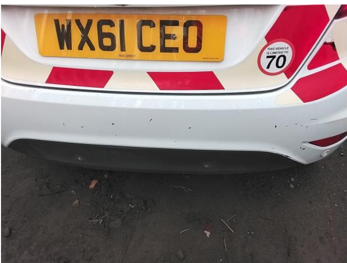
7: Bumper Rear Chipped Multiple Chips
