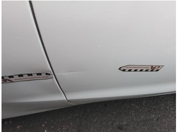
10: Door osf Dented With Paint Damage
