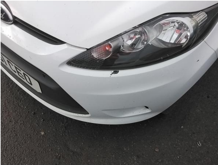
3: Bumper Front Scratched 25 to 100mm Thru Paint
