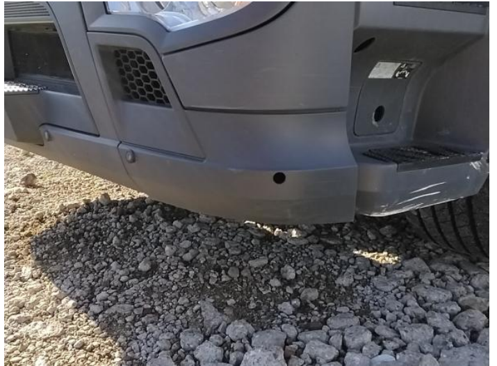
4: Bumper Front Moulding Scuffed (Unpainted) UpTo 100mm
