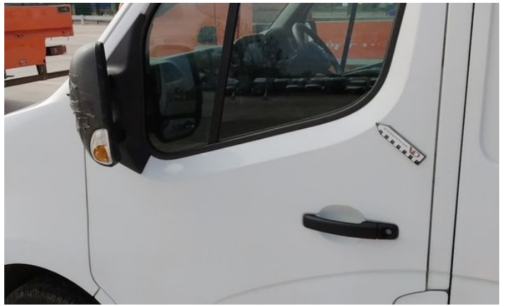
4: Door Mirror Assy nsf Broken Replace
